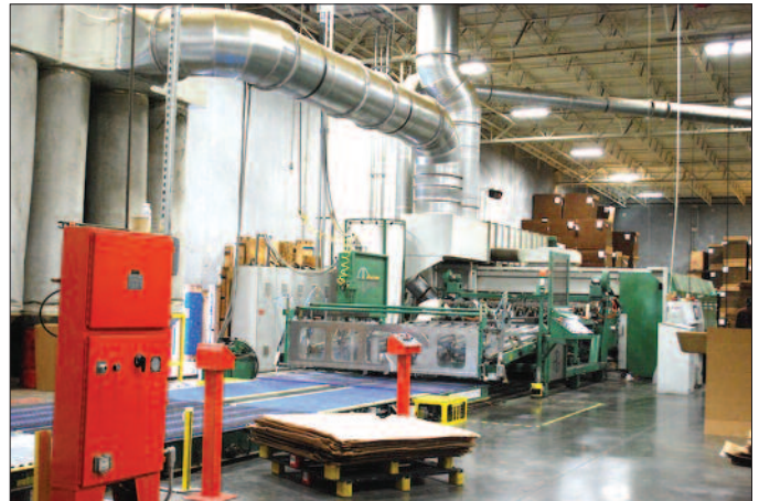
The Martin DRO four-color rotary diecutter was purchased prior to the relocation to drive growth in graphics packaging.
